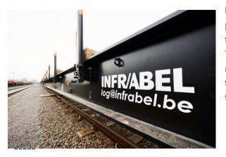
Last April, the first stage of this investment programme was completed with the delivery of the first 12 wagons to the Bascoup workshop. The new cars are 25 metres long, compared to 18 metres for the old ones, and will allow the longer track equipment elements to be transported to their places of use in a more ergonomic manner.
